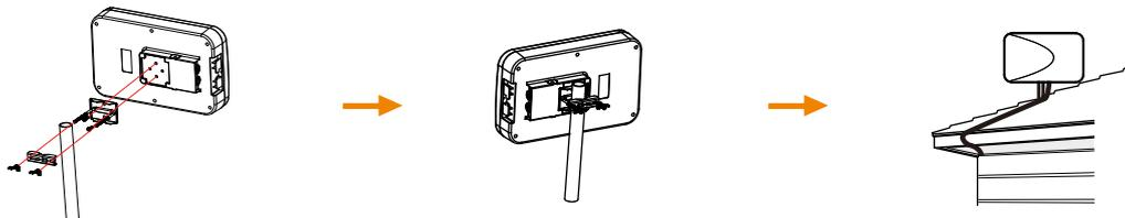
**(Fig.3)** Using the pole mounting accessories to fix the antenna on the balcony.
