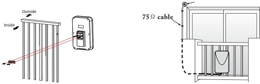
**(Fig.4)** connect the “F” male connector of the coaxial cable to the “F” female connector of the antenna, and wear the water-proof cap to the end of the connected “F” connector.
