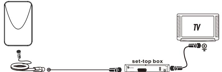
**Installation 2: Connected Through set-top-box (Fig.6)**
