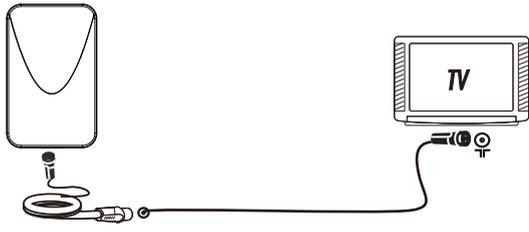
**Installation 1: Directly connected to TV(Fig.5)**
