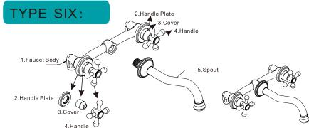
Note: No need to disassemble 2,3,4 parts before fixing it, and make sure there is no silt in water pipes.
