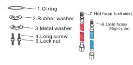
1.Screw the long screws(4) on the faucet. Place o-ring(1) below faucet and screw the hot hose(7),cold hose(6).
