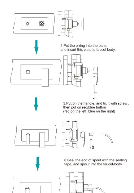
**7**.Installation completed. Open the handle and check whether the function is good.
