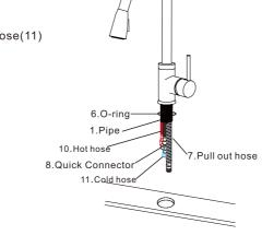
II.Screw rubber washer(2), metal washer(3) and lock nut(4) onto the pipe(1).
