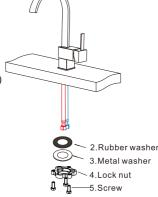
III. Open the hot and cold water supplies. Check for leaks. Turn on faucet handle for one minute to flush debris from faucet
